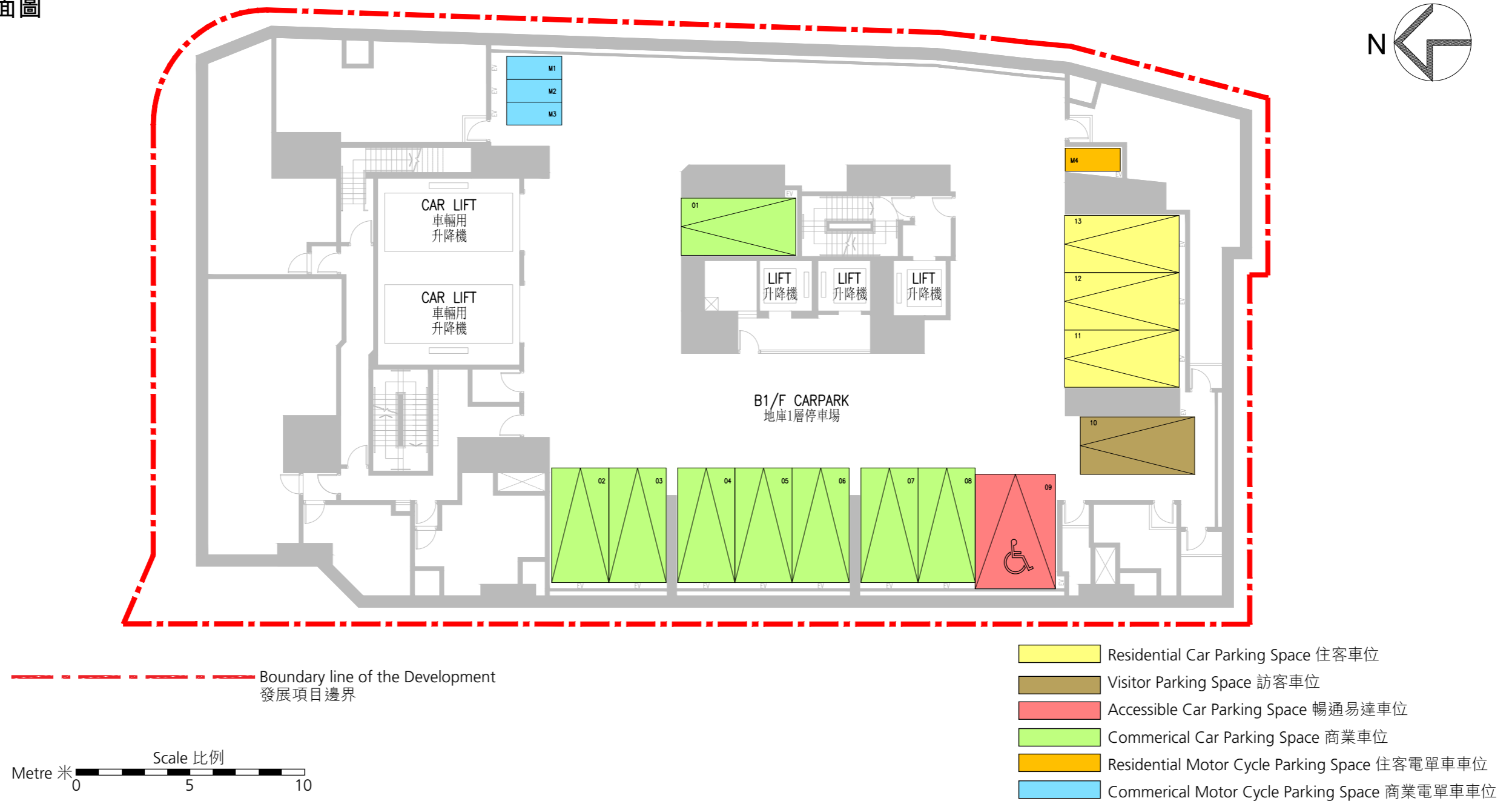
Number, Dimensions and Area of Parking Spaces on B1/F 地庫1層停車位的數目、尺寸及面積
